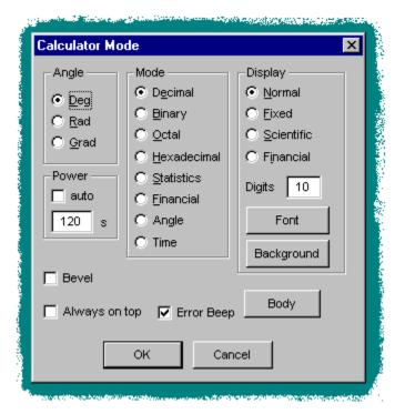
Selecting one of the options in the *Angle* group determines how values of angles are interpreted when using the trigonometric functions.
